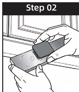
Attach the blue side of the metal sheet to the magnet mark on the rear of the lamp
