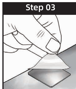
Tear off the white adhesive film on the metal sheet
